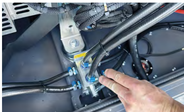
3-way valve for external tank connection
