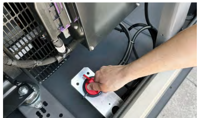
Lockable battery isolator used during maintenance and storage
