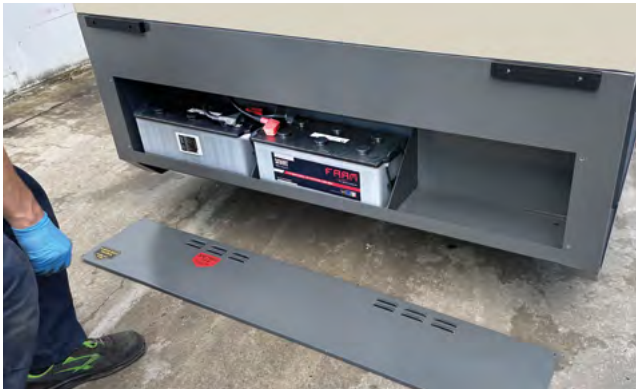
Battery compartment externally accessible for easy maintenance
