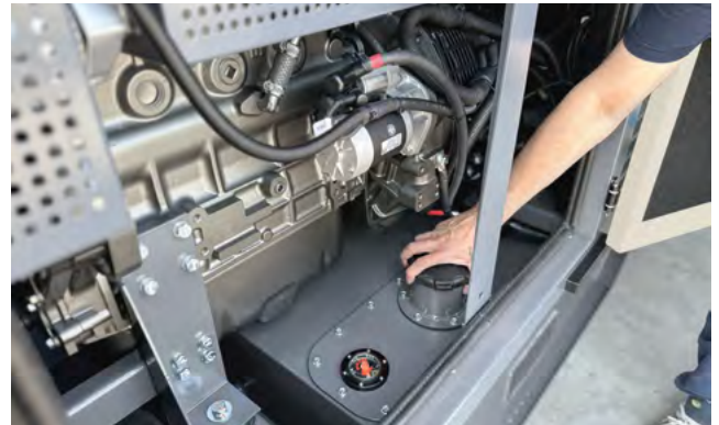
Tank filler with wide tank refilling point
