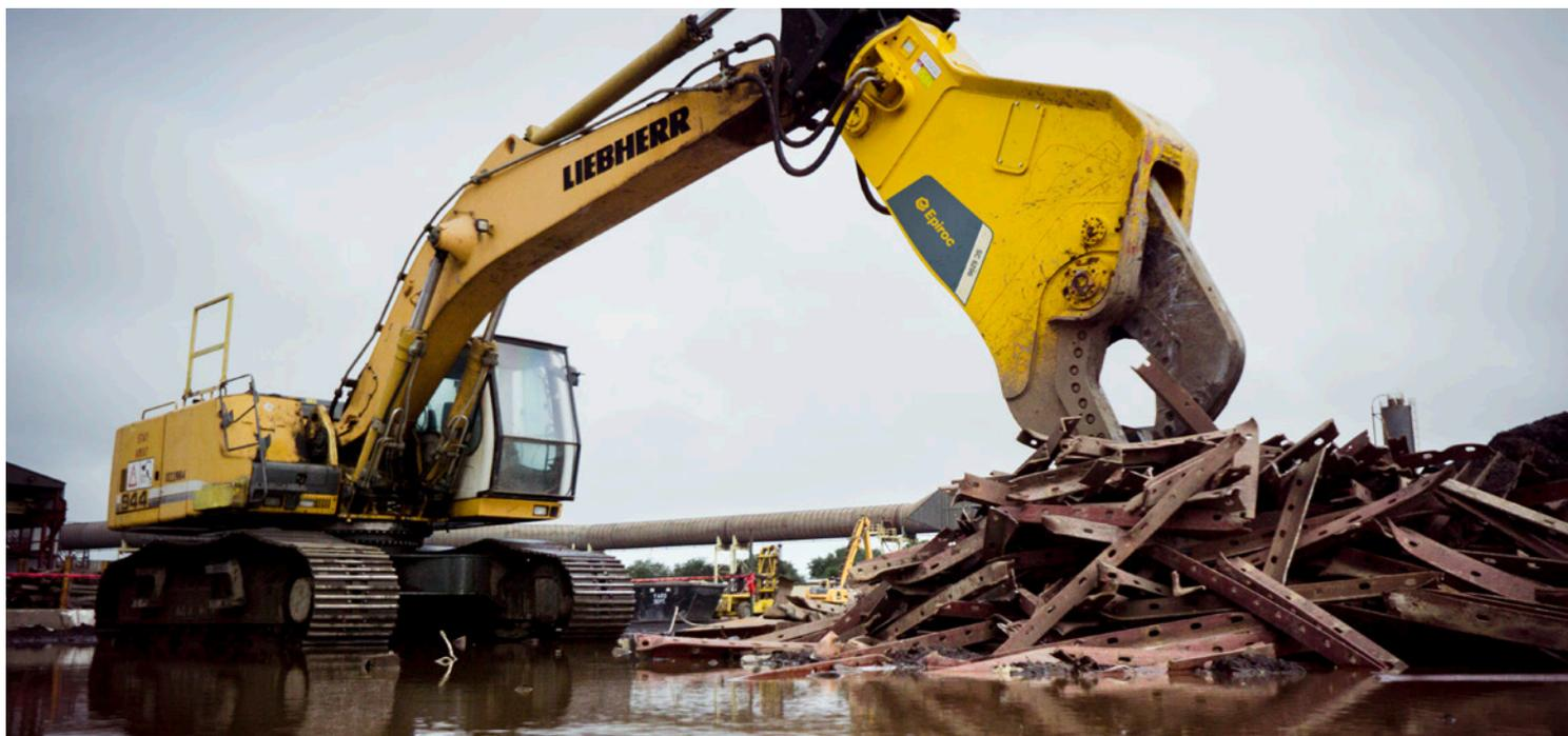
By forcing the material to where the cutter exerts the greatest force, the optimally-shaped jaw cuts through steel easily, no matter the size.
