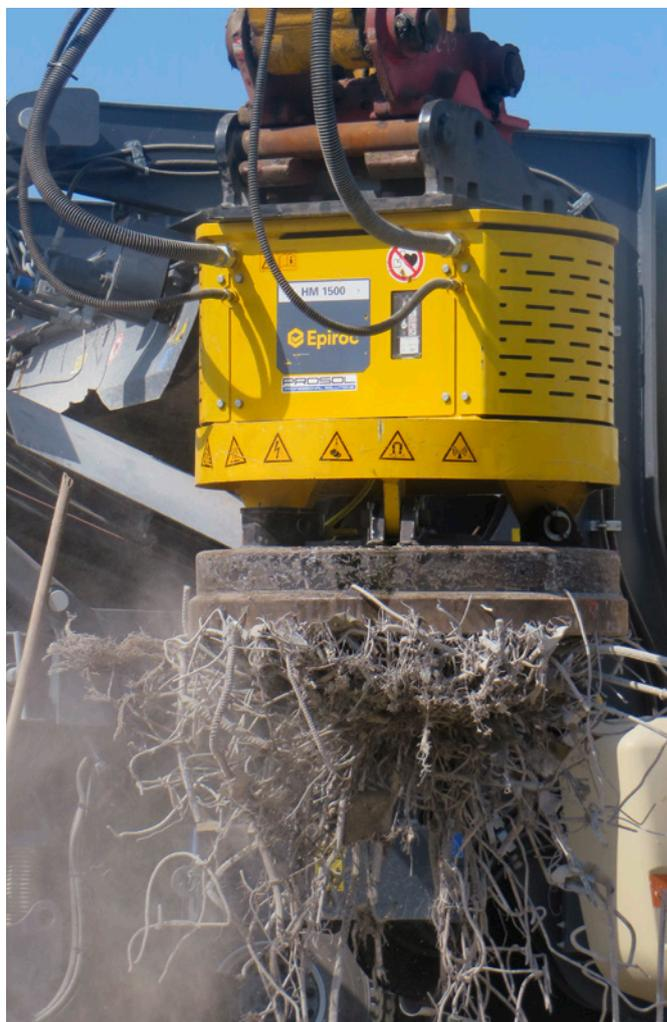
Easy installation makes the Hydro Magnets ideal for demolition sites, scrap yards and recycling facilities.
