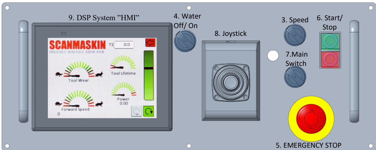
Figure 4-3 Control panel of SCANMASKIN 32 WS RC
