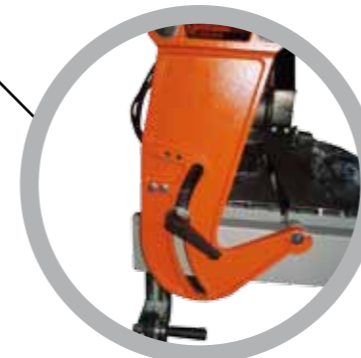
cutting head adjustable up to 45°
