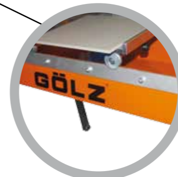
exchangeable guiding rails of cutting table
