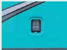
Hydraulic oil tank gauge
