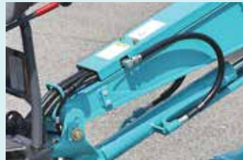
Protective cover for hoses behind the boom
