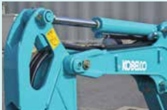
Bucket cylinder hoses sited within the arm
